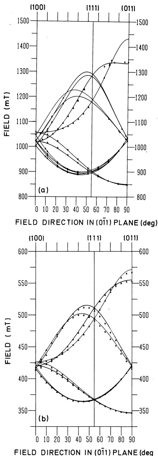
FIG. 6. (a) Result of the fit of spectrum 1 together with the fitted data points. (b) Simulation of spectrum 1 at 9.3 GHz with the parameters listed in Table IV. The data points of Callens *et al.* (Ref. 27) are also shown.
