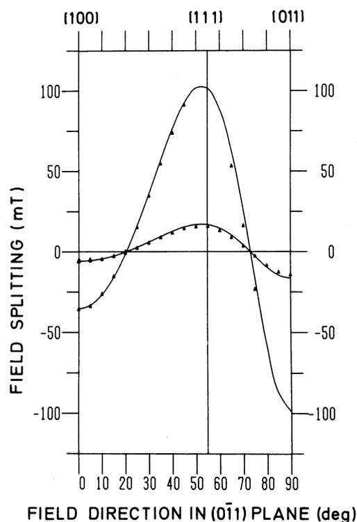
FIG. 7. Splitting of the two lines with the double crossing as fitted in *K* band and simulated in *X* band together with the experimental points.
