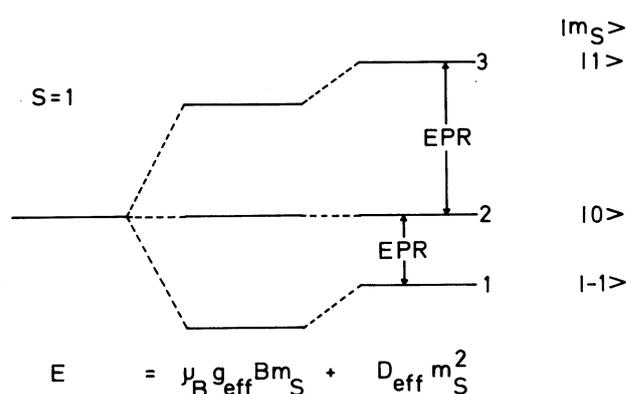
FIG. 5. Schematic energy-level diagram for an  $S=1$  system. The allowed EPR transitions are indicated.
