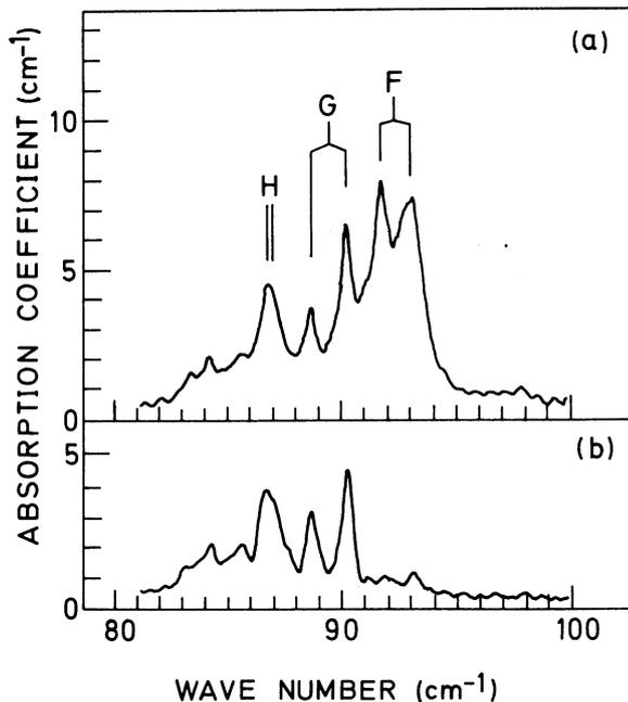
FIG. 1. Absorption spectrum of the annealed sample,  $1s \rightarrow 2p_0$  lines: identification of thermal donors  $F$ ,  $G$ , and  $H$  according to line positions given in Table I. (a) cooling under illumination and (b) cooling in the dark.
