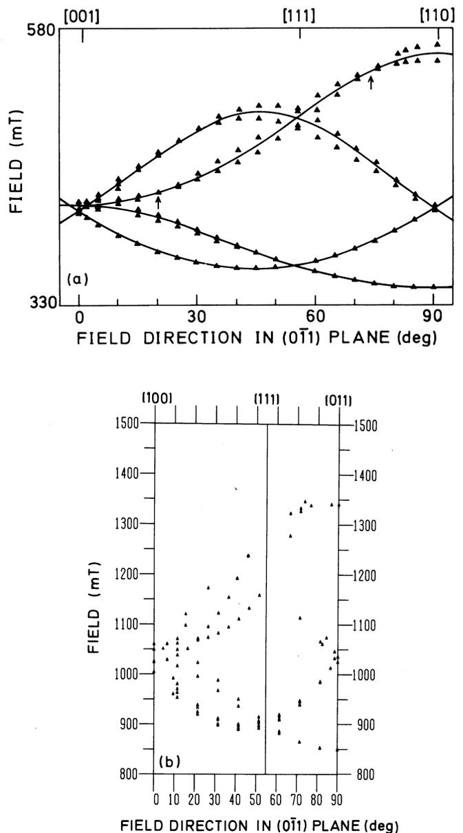
FIG. 4. (a) EPR data points of Callens *et al.* (Ref. 27), together with the averaged  $C_{2v}$  fit of spectrum 1. The measuring frequency was 9.3 GHz. (b) EPR data points as measured at the  $K$  band for spectrum 1. The sample was cooled under illumination. The measuring temperature was 1.6 K and the frequency was 22.800 181 GHz.
